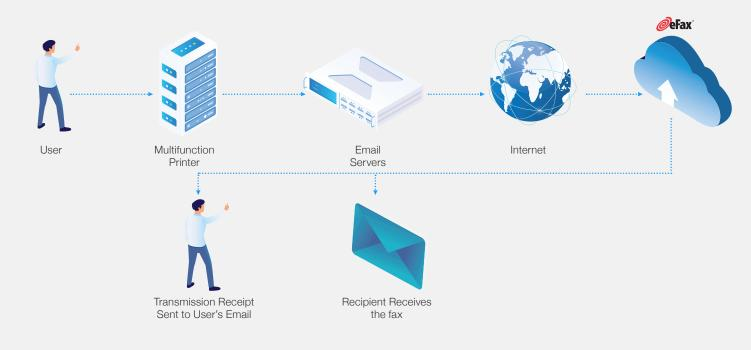
The above scenario represents one of several options for sending a cloud-based fax directly over the Internet using your standard office MFP. With a versatile and flexible enterprise service such as the one from eFax, you will have several MFP integration options available, which you can choose based on your company's existing network architecture and faxing needs.
